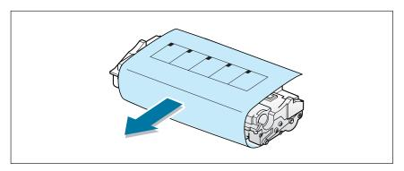
3. Shake the cartridge from side to side 5 or 6 times to redistribute the toner evenly inside the cartridge.
